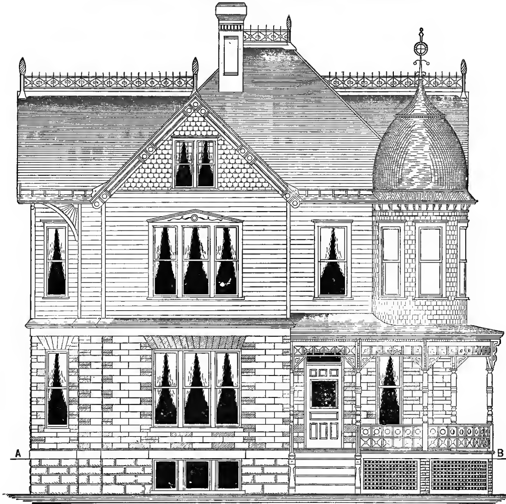
Fig. 38.—Front Elevation, Showing Method of Shading, etc.—Scale, \frac{1}{8} Inch to the Foot.
